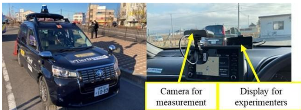
FIGURE 6.14 The automated driving vehicle, the display for experimenters and the camera for measurement
