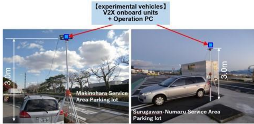
FIGURE 6.19 Picture of vehicle with V2X unit V2X Antenna for OBU is used for roadside units and the characteristics are not optimized
