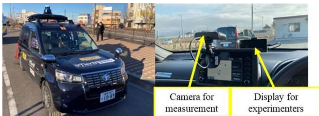
FIGURE 7.14 The automated driving vehicle, the display for experimenters and the camera for measurement
