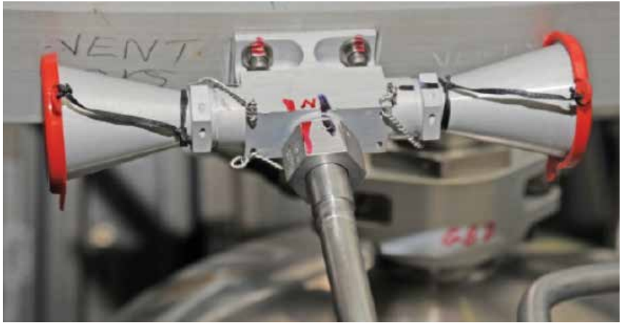
Figure 1.9: Oppositely oriented nozzle configuration ensures equal thrust in opposite direction and no orbital change
