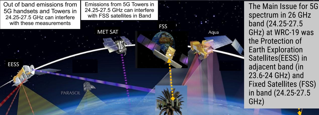
H<sub>2</sub>O Molecular absorption peak in 23.6-24 GHz Key to accurate measurement of the vertical water vapour content
