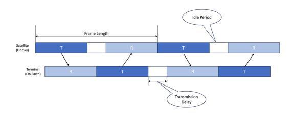
The row on the top of the figure is the frame that is linked to the MSS satellite that is located up in the orbit. Here "T" represents the period where the MSS satellite is transmitting and "R" is the portion of the frame where the satellite is receiving. The period between these two blocks sandwiches an idle period when the satellite is doing nothing because this is the time the RF signal takes to reach the terminal located on the ground, and its transmission reaching back to the satellite.
