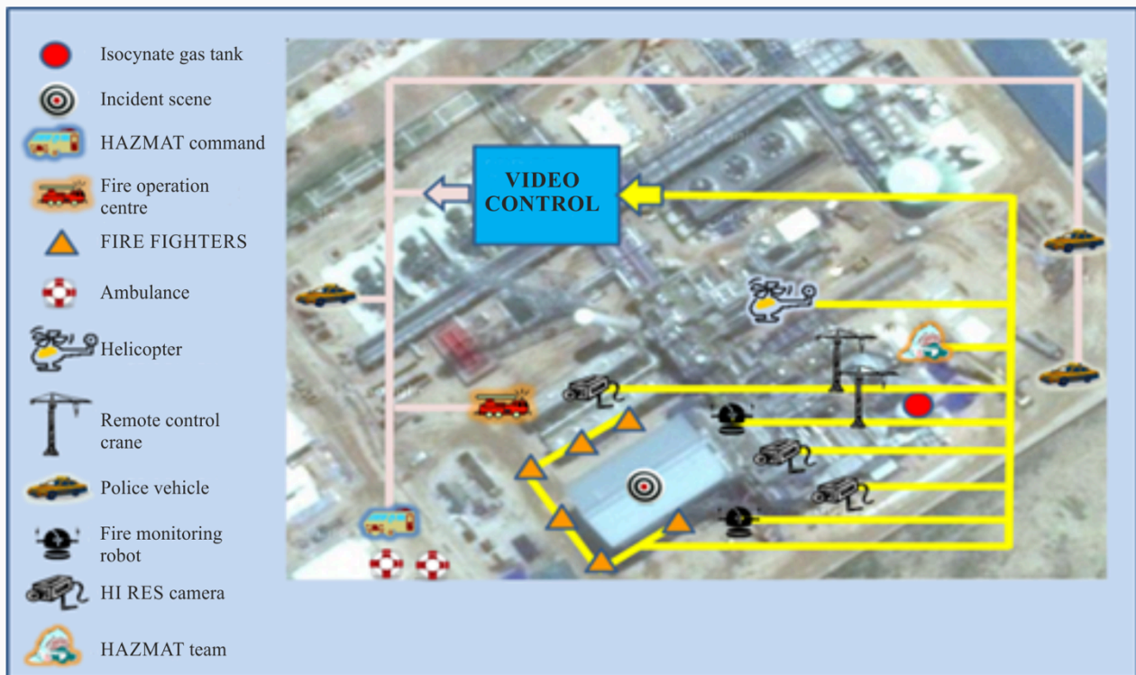
FIGURE 3 Deployment of various resources
