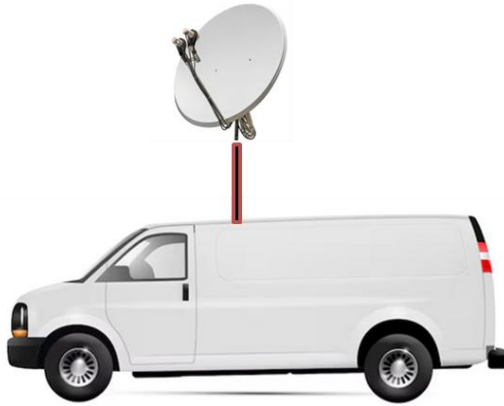
FIGURE 2 Single satellite cell pfd measurement set-up
