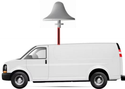
FIGURE 1 Aggregated pfd measurement set-up
