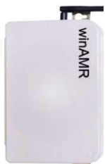
Router/ Signal Booster
